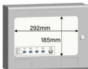
Max. number of LED's = 40 Will house 1 x 8 Red LED driver PCB and 2 x 16 LED extension PCB's (Red, Green or Yellow) 369mm wide x 310 mm high x 90mm deep
